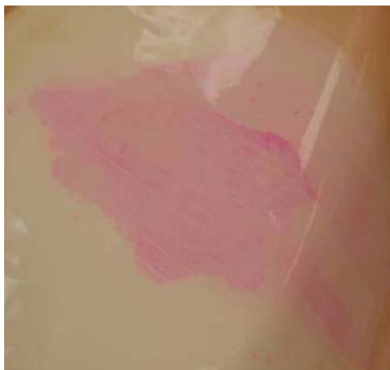
Figure 3 Dye Test on oxidised membrane
